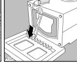
Repeat the operation for the right polythene bag, removing it towards the left and then upwards.
